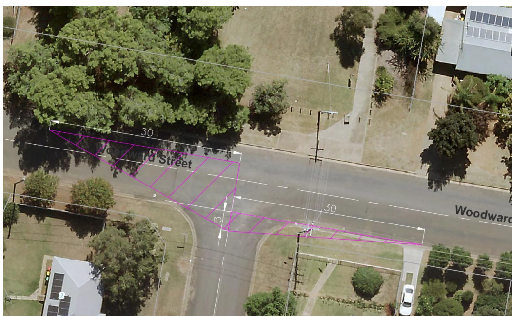
Figure 4 Sight distance analysis for the intersection of Woodward and Fisher streets
