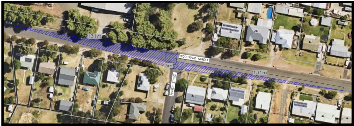
Figure 3: Sight Distance Analysis for the GIVEWAY Intersection of Woodward and Fisher Street
